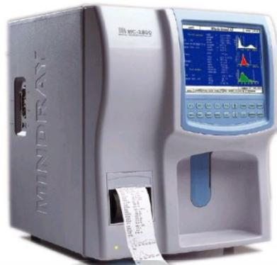
Gambar 4. BC-2600 Auto Hematologi Analyzer (Mindray, 2006).
