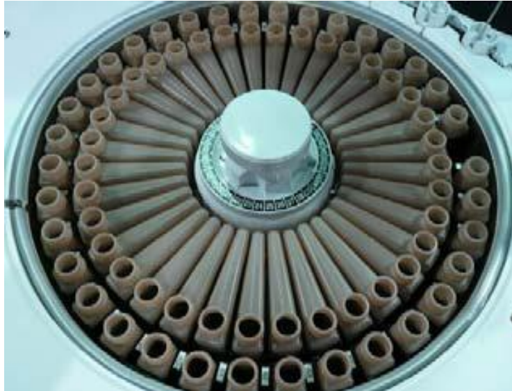
Gambar 2. Tray Reagen alat kimia analyser TMS Superior 50i.(Dikutip : Medsys Inc.2016)
