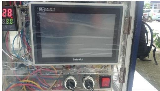
**Gambar : 3.11** *Autonics Graphic Panel GP-SO70*
