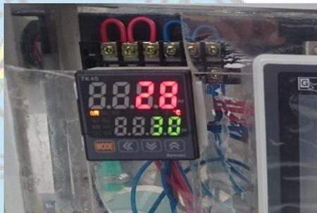
**Gambar : 3.13** Digital *Temperature Controller* TK 4S
