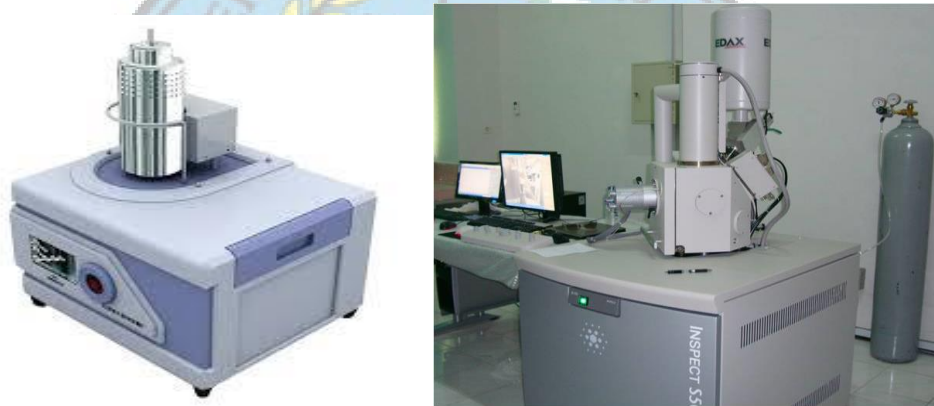
Gambar 2.16. Alat uji Thermo Gravimetric Analyzer ( centrallaaboratory.umac.id )
