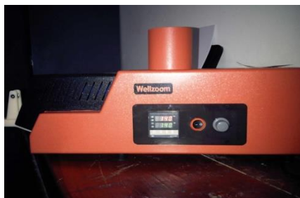
Gambar 3.7. Mesin screw extrusion filamen print 3D (dokumentasi, 2016)
