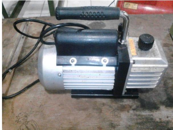
Gambar 3.2 Pompa Vakum
