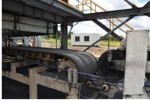
Gambar 2.27. Cable Belt Conveyors
