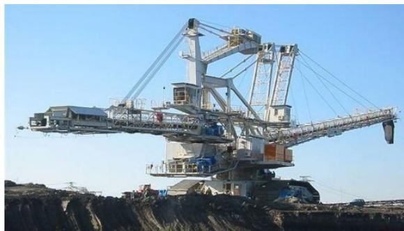
Gambar 2.29. Mobile Transfer Conveyors
