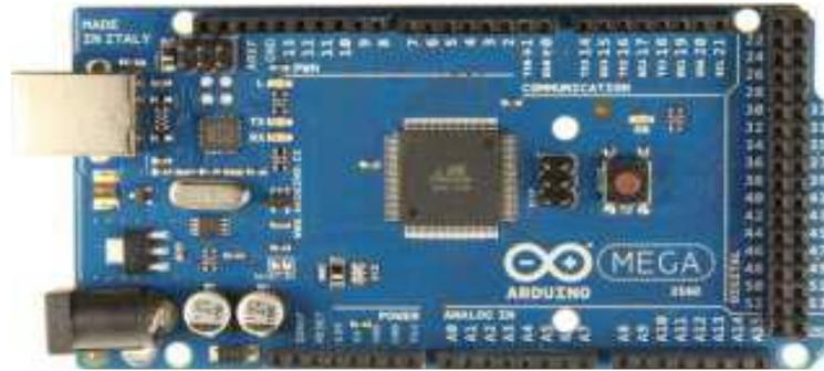
Gambar 2.19 Arduino Mega 2560
