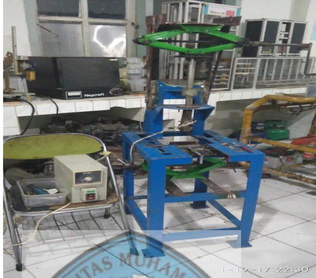
**Gambar 2.10** Alat *Injection Molding*
