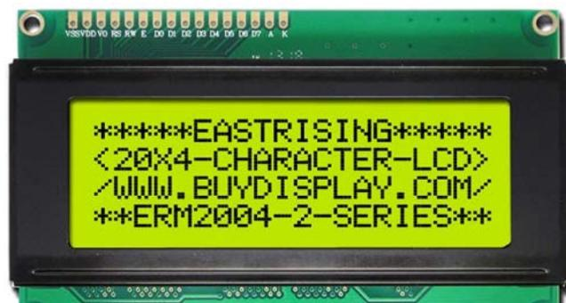
**Gambar 2.11.LCD (Liquid Crystal Display)20 Karakter 4 Baris ERM2004SYG-2
