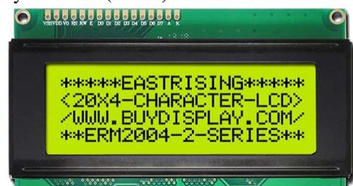
**Gambar 2.11.LCD (Liquid Crystal Display)20 Karakter 4 Baris ERM2004SYG-2 (Datasheet LCD (Liquid Crystal Display) ERM2004-2)**
