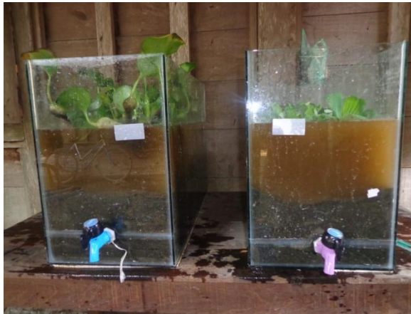
Bak Subsurface Flow Wetland
