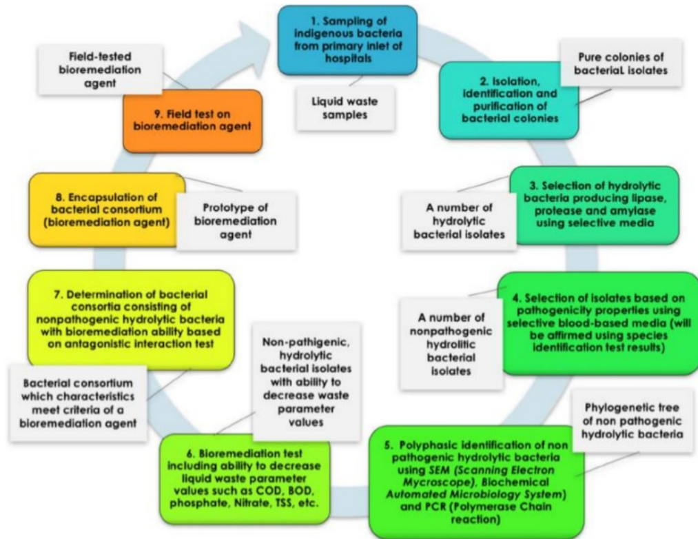
Fig. 3 More detailed scheme of steps required to obtain bioremediation agent from groups of hydrolytic bacteria isolated from hospital liquid biomedical waste reservoir and the targeted outcomes of each step
