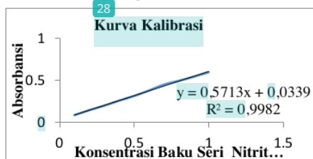
Gambar 3. Kurva Kalibrasi Larutan Baku Seri Nitrit 0,1 – 1,0 ppm
