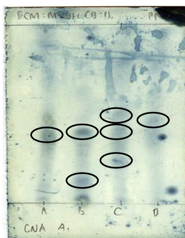
Figure 4. Diagrammatic chromatogram crude extract of Actinomycetes samples of CNA 148 with PMA reagent using DCM : methanol (90:10) solvents.
