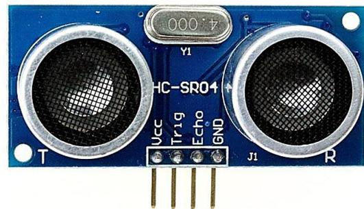
Gambar 2. Sensor Ultrasonik HC-SR04
