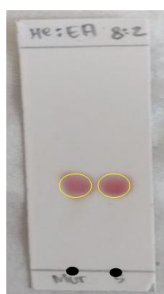
Figure 1. TLC analysis of MCE5 (left) against \beta -sitosterol standard (right). Both showed similar Rf values.
