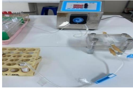
Gambar 8.2 Prototype alat hemodialisa (Mukaromah, Soraya, & Ariyadi, 2022)
